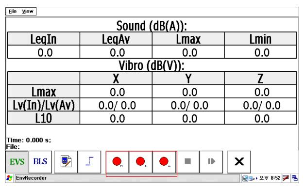
16. The saved data will be stored in the SD memory cad, you can move the saved data of the SD memory card to your PC, and you can analyze the data with the PC EVS analysis software.
