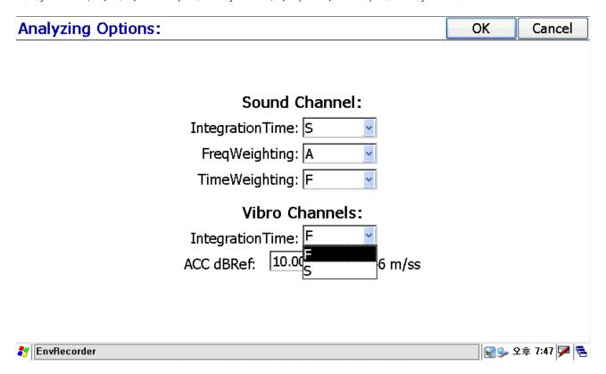
[Example] Vibro Channels-IntegrationTime: Set up Integration time for the vibration channels. F(Fast) has 100ms of integration time, S(Slow) has 1 sec of Integration time.
