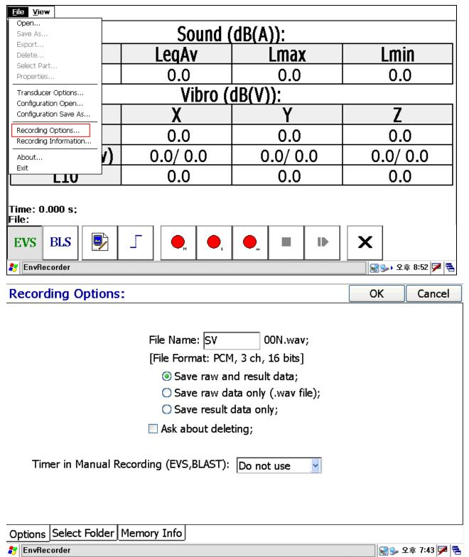
9. Select "Folder" at the bottom in the "Recording Options", and select the position to save the file. The data has to be saved in the SD Memory by our program.
