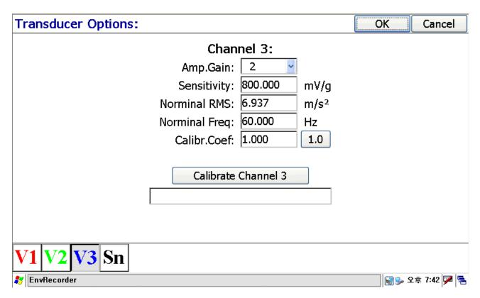
7. "Please put the sensivity of the microphone for the Sn" (Channel 4), and connect the sound calibrator with 94dB output at 1kHz to the microphone, and generate standard signal, and click "OK" to move measurement window, and check the measuring value, please put "Calibra. Coef" value to be corresponded with that Leq value is 94dBw. If you finished all channels, please click "OK" to exit.
