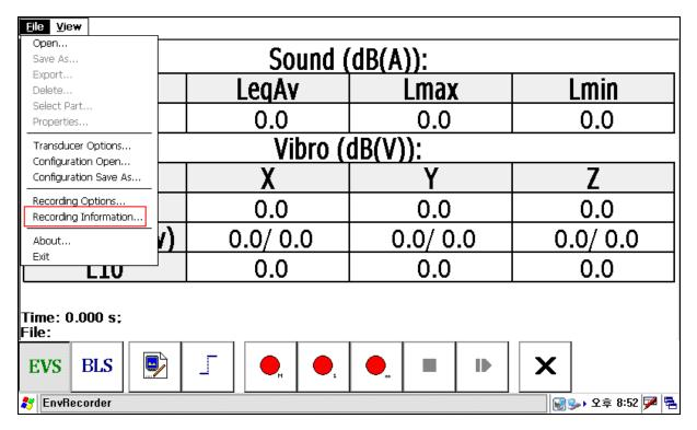
(2) Put the saving information for the data. Name of person, Object of measurement, measuring position, Axis direction information of 1,2,3 channels for vibration name.
