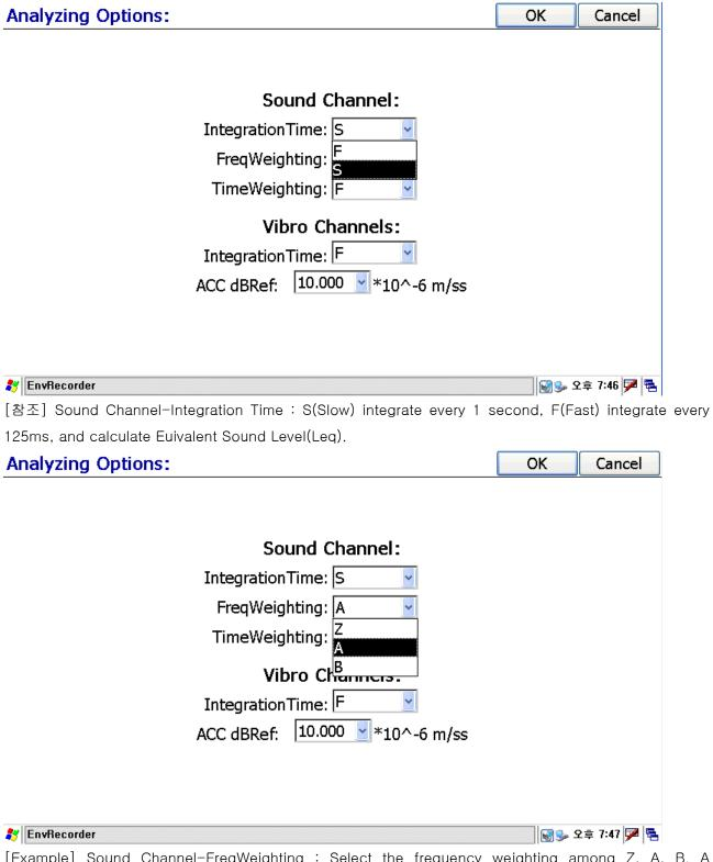
[Example] Sound Channel-FreqWeighting: Select the frequency weighting among Z, A, B. A frequency weighting is designed to meet with human ear.
