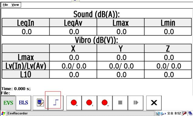
11. Move "Trigger Options" window, and set up "trigger level" with dB by "Vibration RMS", and select "Recording Time". You can select "Trigger Level" by 1 dB step from 45dB to 60dB, Recording Time can be selected among 1s, 2s, 3s, 5s, 10s, 1min, 5min, 1hour. Please click "OK".
