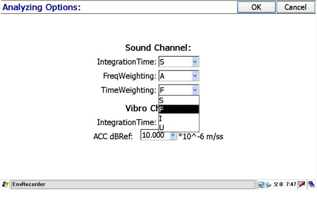
[Example] Sound Channel-TimeWeighting: Time weighting is weighted by time F(Fast) is sampled every 125ms, S(Slow) is sampled every 1 sec, I(Impulse) is sampled every 35ms.
